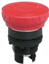
Automatic Push/Turn Mushroom. Manual push "In" Latches "In". Turn clockwise to unlatch. Spring return.
