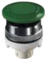
Automatic Push/Turn Mushroom. Manual push "In". Latches "In". Turn clockwise to unlatch. Spring return.
