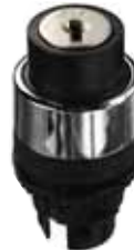
Key Twist 90° Maintained. (PS-T3K-B) Turn key clockwise to latch "In". Turn key counterclockwise to release. Key withdrawable in both positions. Black only.
